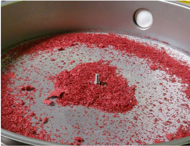
Figure 3. The Russell Eco Separator® separating dust and seeds at Eco Treasures
