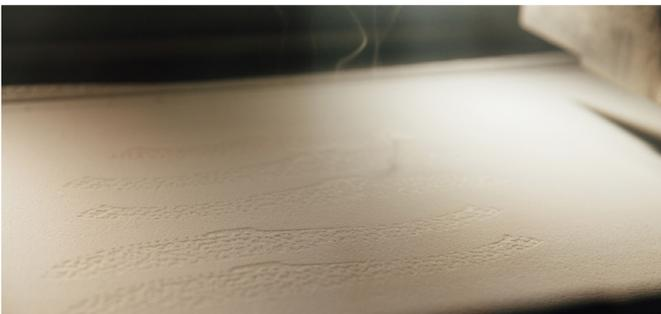
**Figure 2.** Selective laser sintering used to produce midsole
