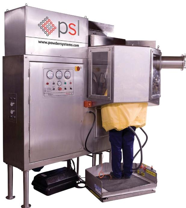
**Figure 2.** The PSI high containment isolator
