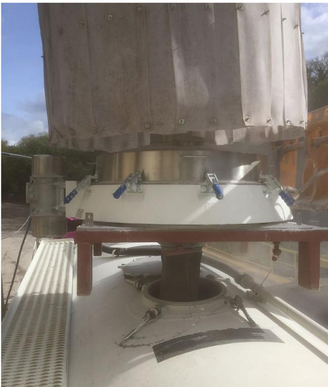
**Figure 2.** The Russell Compact Sieve® guarantees the quality of powders during tanker loading
