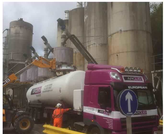
**Figure 1.** The Russell Compact Sieve® used to check-screen marble powder during loading of delivery tankers
