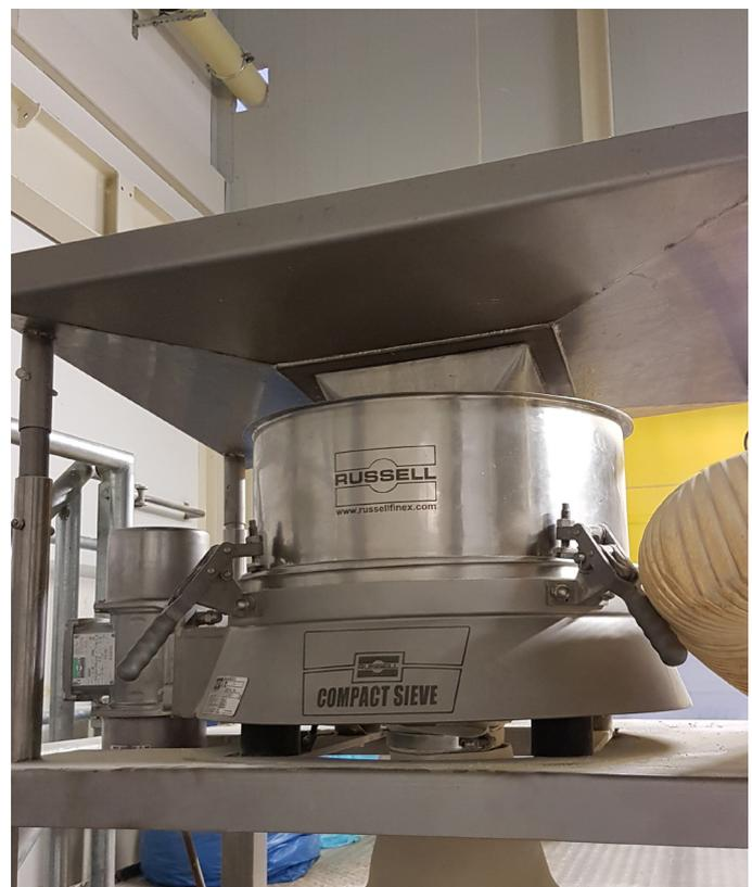
**Figure 1.** The Russell Compact Sieve® installed on site at Lactoprot's facility in Lübeck
