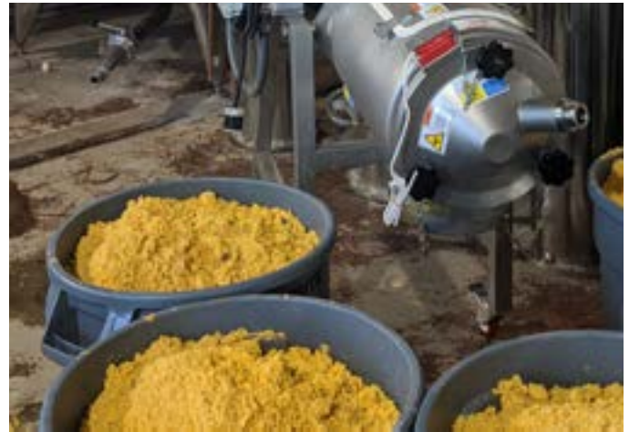
Figure 2. An example of the spent grains used as animal feed separated out by the Liquid Solid Separator™
