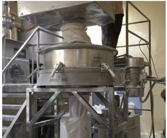
**Figure 1.** The Russell Compact Sieve® installed to screen pharmaceutical powders at Sri Krishna Pharma's Uppal factory
