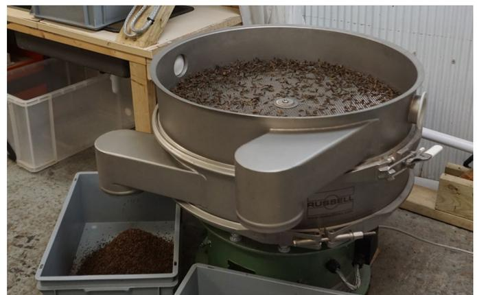
**Figure 1.** The Russell Eco Separator® is used to separate the black soldier fly larvae from the frass
