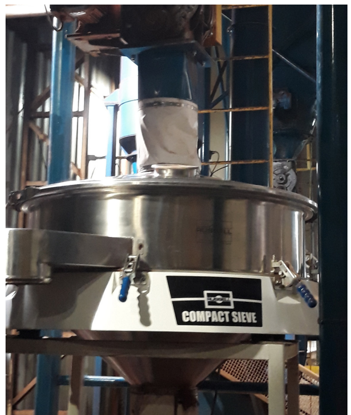
Figure 1. The Russell Compact Sieve® is used to remove contamination from cocoa product at the IBC factory
