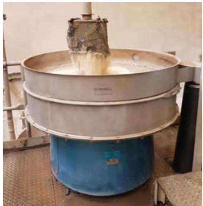
**Figure 1.** The Finex Separator™ is installed at PFR Nord to separate the solids from the wash water
