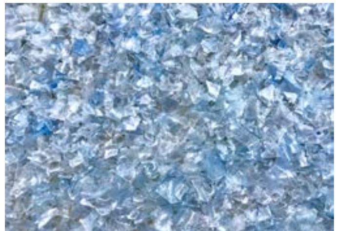
**Figure 2.** An example of the ground PET plastics PFR recycle and separate with the Finex Separator™
