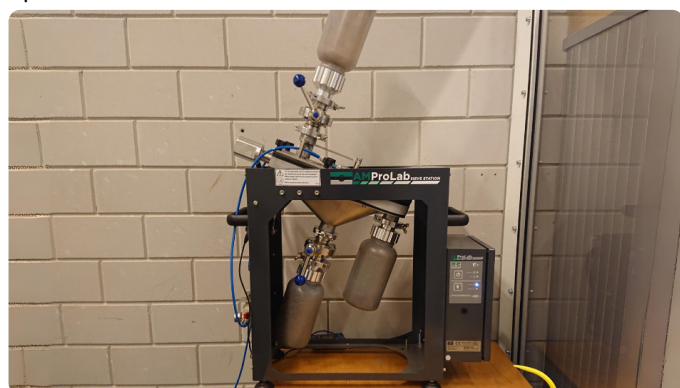
The Russell AMPro® Lab Sieve Station installed in UvA's Faculty of Science
