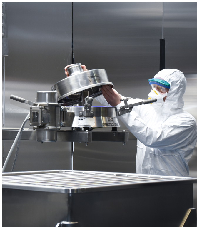
Figure 4. The Russell Compact Sieve® is quick and easy to dismantle and clean
