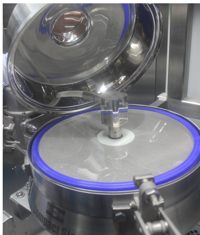
Figure 3. The all-stainless steel Russell Compact Sieve®
