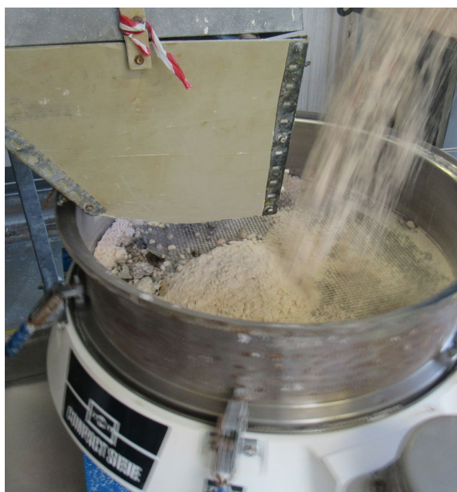
Figure 1. The Russell Compact Sieve® installed as part of a conveying line for incoming raw materials at Kemira Chemicals (UK) Ltd.
