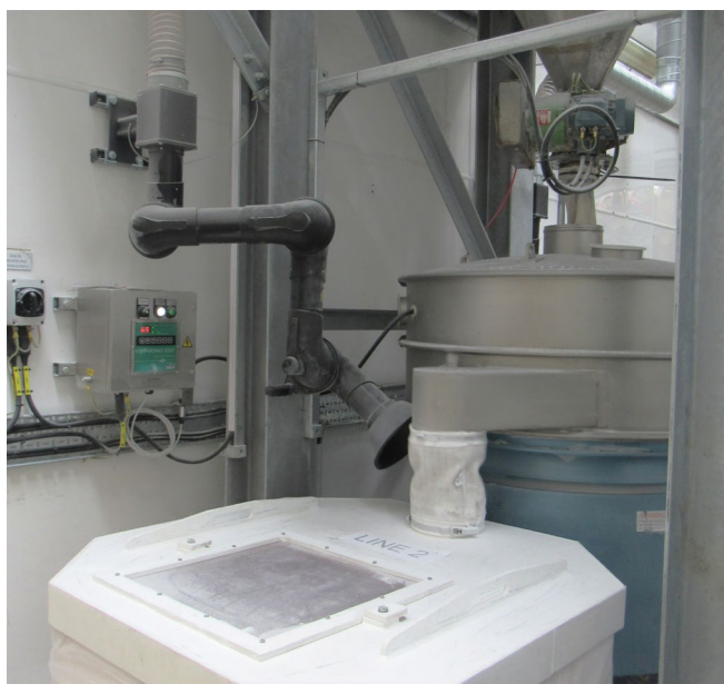
Figure 2. The Finex Separator™ has significantly enhanced the sieving capacity of the polymer beads production line
