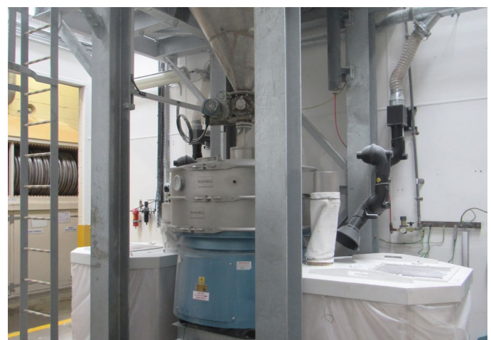
Figure 1. The Finex Separator™ with Russell Vibrasonic® Deblinding System installed at Lucite International Group Ltd to ensure accurate sizing of polymer beads
