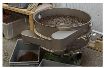
**Figure 1.** The Russell Eco Separator® is used to separate the black soldier fly larvae from the frass
