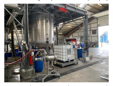
the liquid into a blending tank along with extra ingredients for further conditioning. After a quality check, the emulsified products are ready for packaging into intermediate bulk containers.
