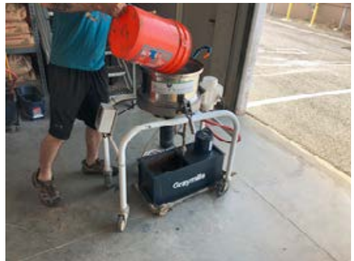
Figure 1. Paleo Solutions using the Russell Mini Sifter™ as a wet screening unit for the gravel matrix
