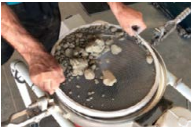
Figure 2. Paleo Solutions using the Russell Mini Sifter™ as a dry screening unit
