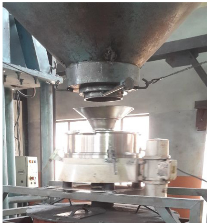
Figure 1. Installation of the Russell Compact Sieve® at Industrial Metal Powders (India) Pvt. Ltd
