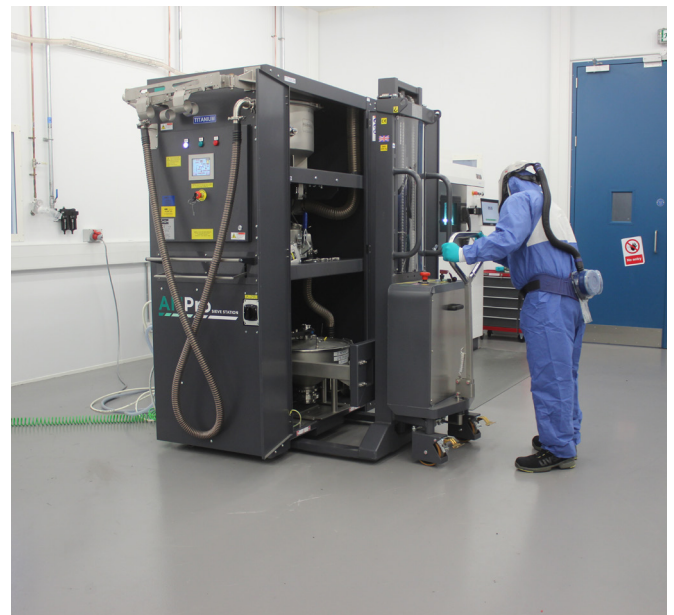
Figure 1. The Russell AMPro® Sieve Station is easy to move, and operate, in order to reuse and reclaim AM powder from the build process.
