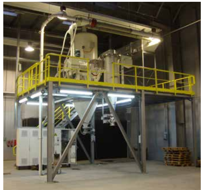
Figure 2: Typical installation supplied by Neuman and Esser with the screening operation commonly positioned under the cyclone prior to the filling lines.
