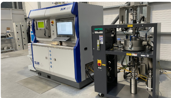
The AMPro® Lite integrated with the SLM280 printer
