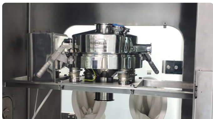
Our Russell Compact Sieve® with side mounted ultrasonic probe
